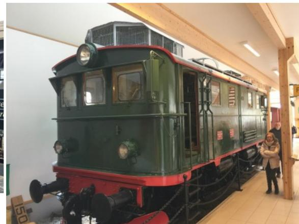
First loco used on newly electrified Flam Railway, vintage 1944. Because of the steep descent of the Flam line, this EL9 was delivered with a special braking system, the first locomotive delivered with electrical resistance brakes. In all, this loco had five different braking systems. Served on the Flam line until 1984.
